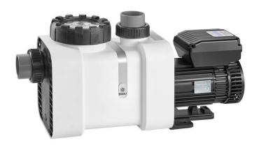
The BADU Delta swimming pool pump has a motor display with intuitive controls, which ensure low energy consumption. It is especially quiet and efficient due to newly configured hydraulics. LED lighting in the transparent lid aids sight inspections. Inset drain plugs avoid risk of breakage. The permanent magnet motor provides efficient energy savings. Can be controlled using the BADU Eco Logic remote control.<br/>
