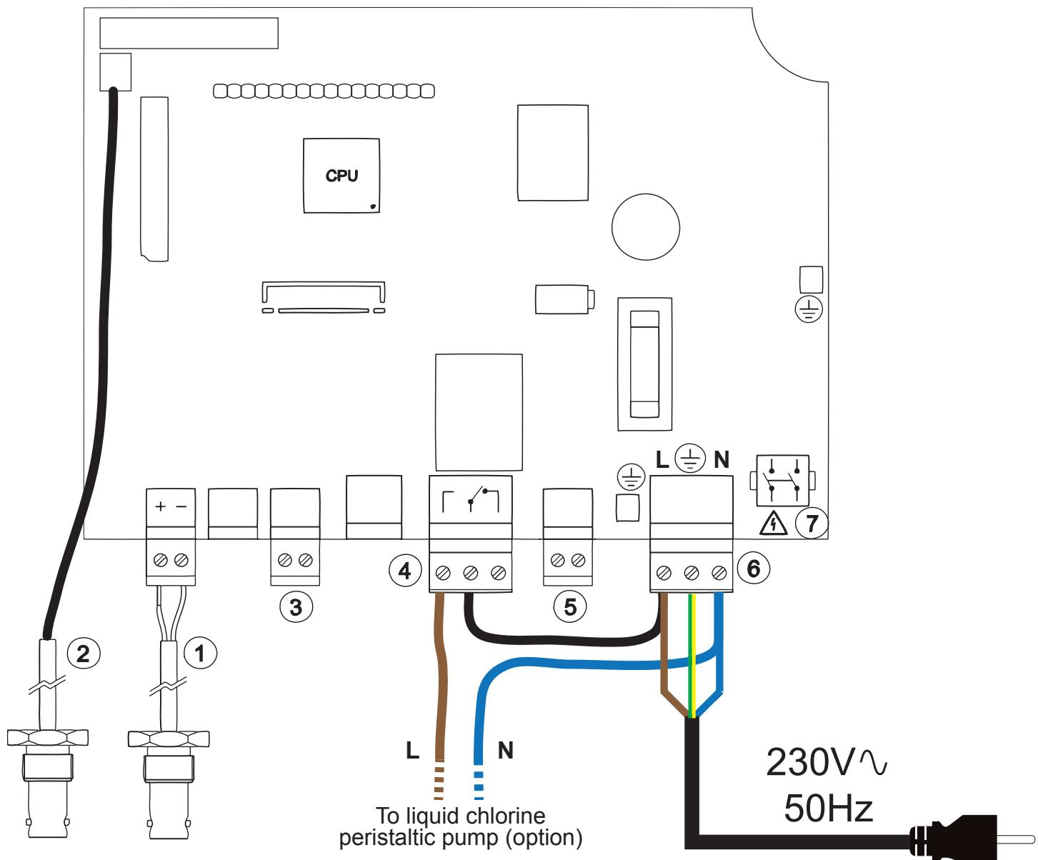
1 BNC connector for the pH probe
