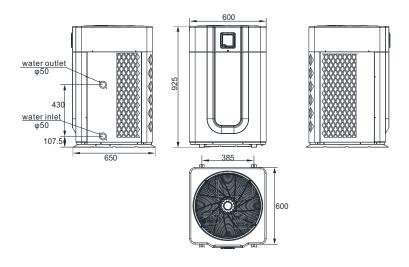
Model:PV 21/PV 24 unit mm
